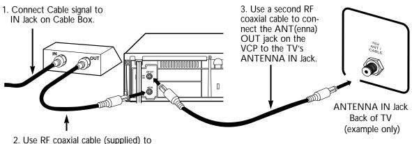
2. Use RF coaxial cable (supplied) to connect OUT Jack on Cable Box to ANT(enna) IN Jack on VCP.
